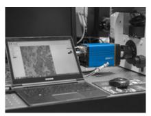
Typical microscope set-up of the pco.flim connected to the camera port of an inverted microscope. The camera is controlled and read out by a computer.
